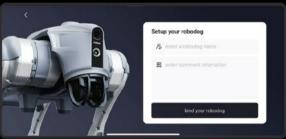
c) Bind the robot: you can choose AP router mode and Wi-Fi connection mode to connect, you can learn the built-in tutorial to quickly master the operation skills after successful connection.
